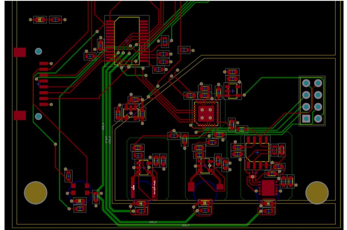
*PCB schematic of the current optical sensor PCB prototype*
