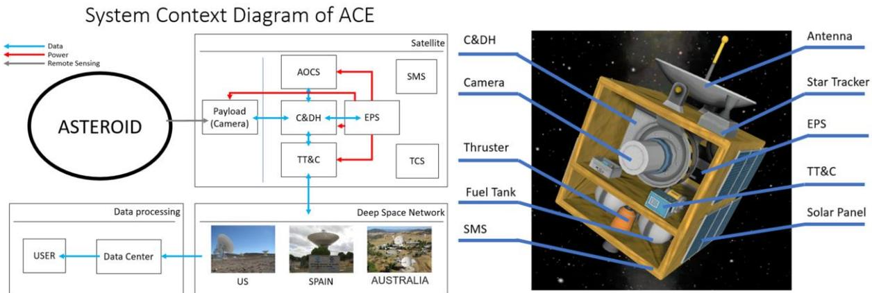
**Figure 4.** A system context diagram of ACE (left) and an illustration of ACE spacecraft layout (right). The system context diagram defines the boundaries and shows the relations between the systems and its environment in the mission.
