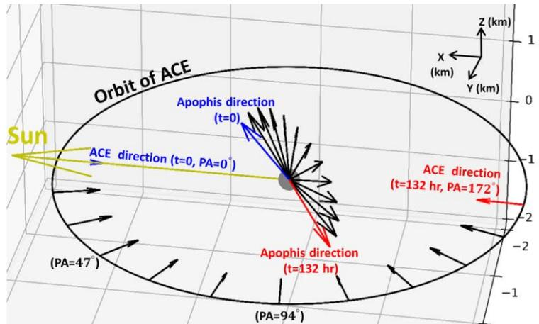
**Figure 3.** The orbit of ACE with the Sun at the direction of +x axis. The arrows indicate the pointing of the imager at a given time (t) and phase angle (PA) as examples. Note that we assume the orientation of Apophis' spin axis in the X-Z plane since it is still unclear due to Apophis' tumbling rotation state [8].
