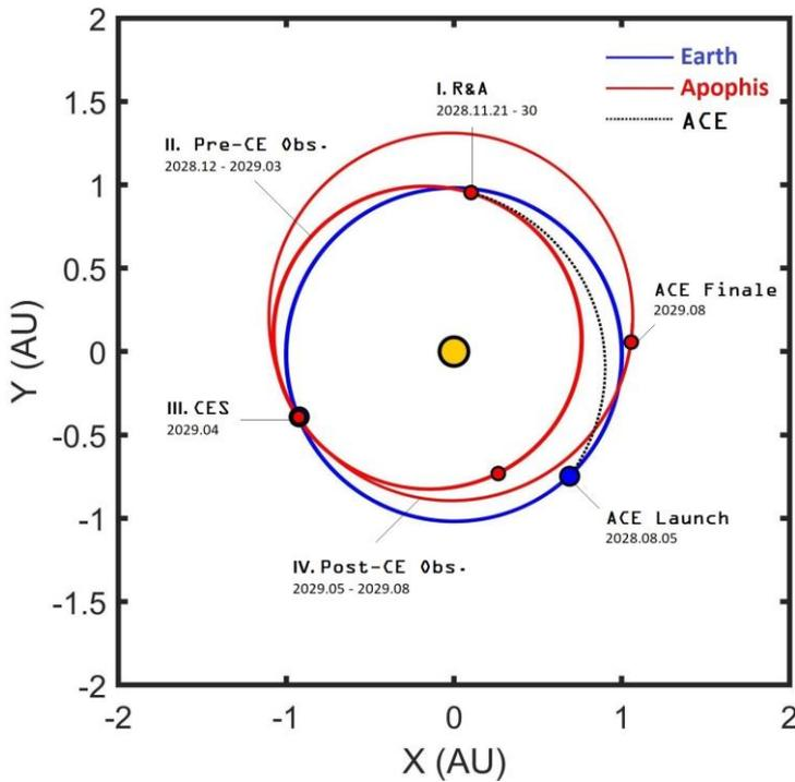
**Figure 2.** The trajectories of Earth (blue), Apophis (red) and ACE (dot) and their relative positions with the corresponding mission stages.
