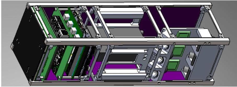
**Figure 3: CAD model of the satellite with external panels removed, showing the EPS, OBC, and transceiver (left unit), spectrometer and magnet mounts (middle), and primary payload (right). Wiring is omitted.**
