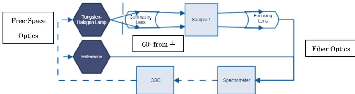
**Figure 2: Block diagram of one optical assembly to observe a sample.**
