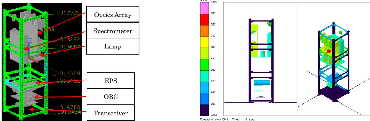
**Figure 5: Payload operation thermal simulation using Thermal Desktop. Critical components are >280 K**
