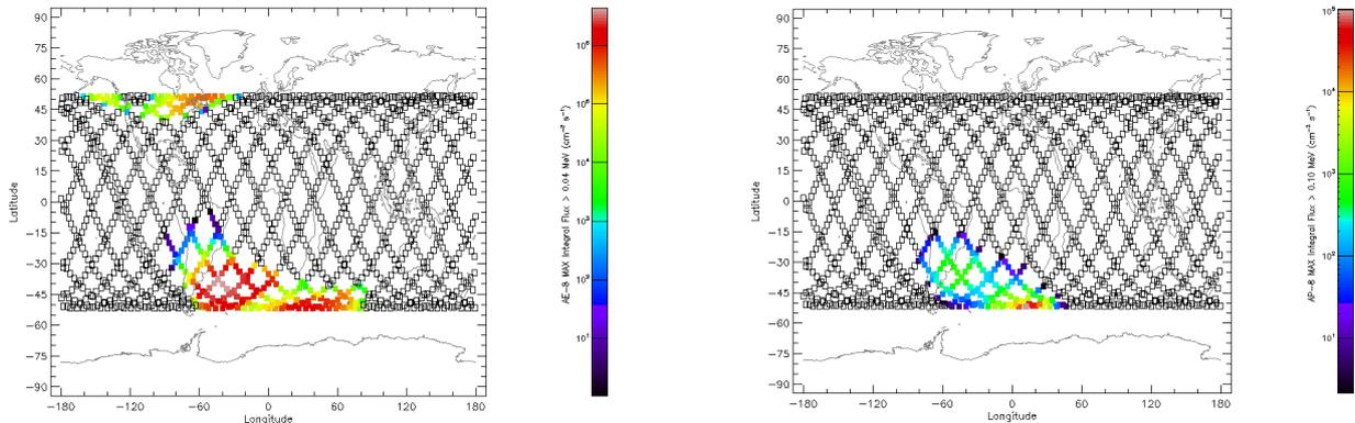
**Figure 4: Maximum electron (left) and proton (right) fluxes expected in ISS flight path over July 2018 using the AE-8 and AP-8 models in SPENVIS respectively. Fluxes range from 10 to 10<sup>5</sup> cm<sup>-2</sup> s<sup>-1</sup> in images.**
