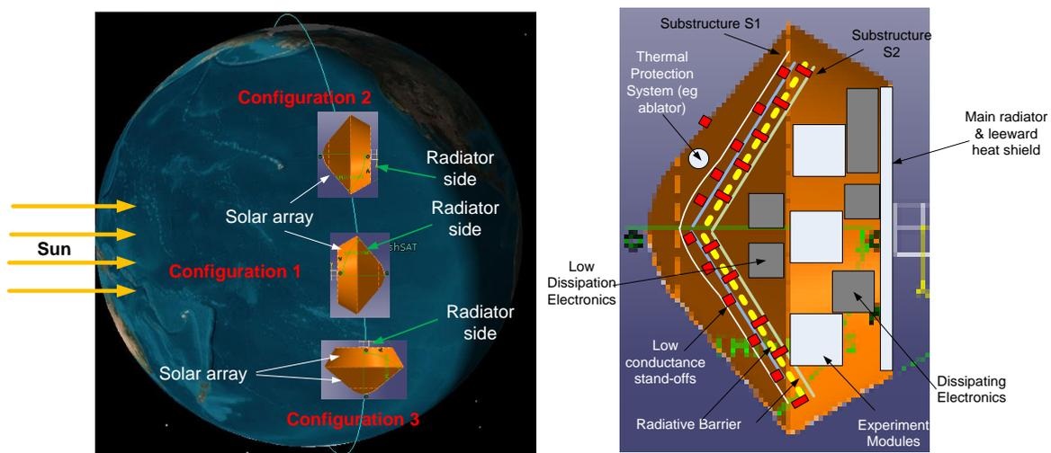
**Figure 2 – MERS flight configurations and internal cut-away view**
