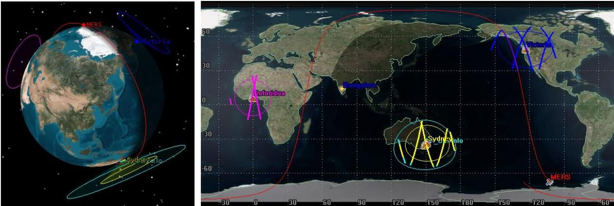
**Figure 3 – Minimum MERS visibility: 3 ground stations and 400km orbit altitude**
