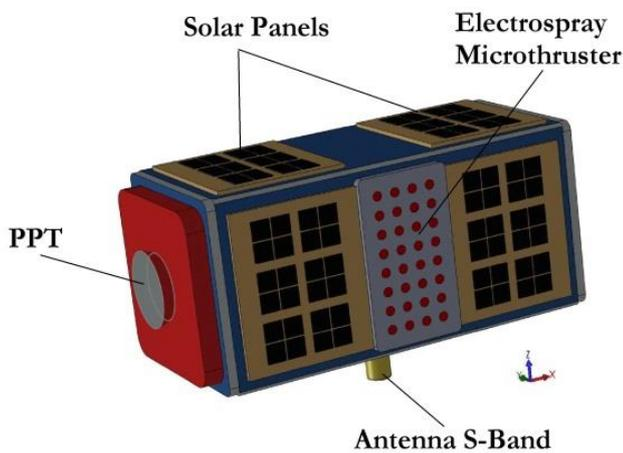
Figure 2. Preliminary CAD configuration.
