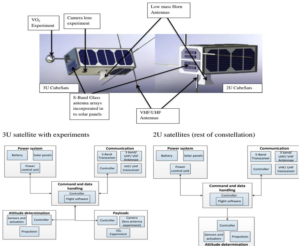
Figure 5.1: 3U and 2U satellite subsystems
