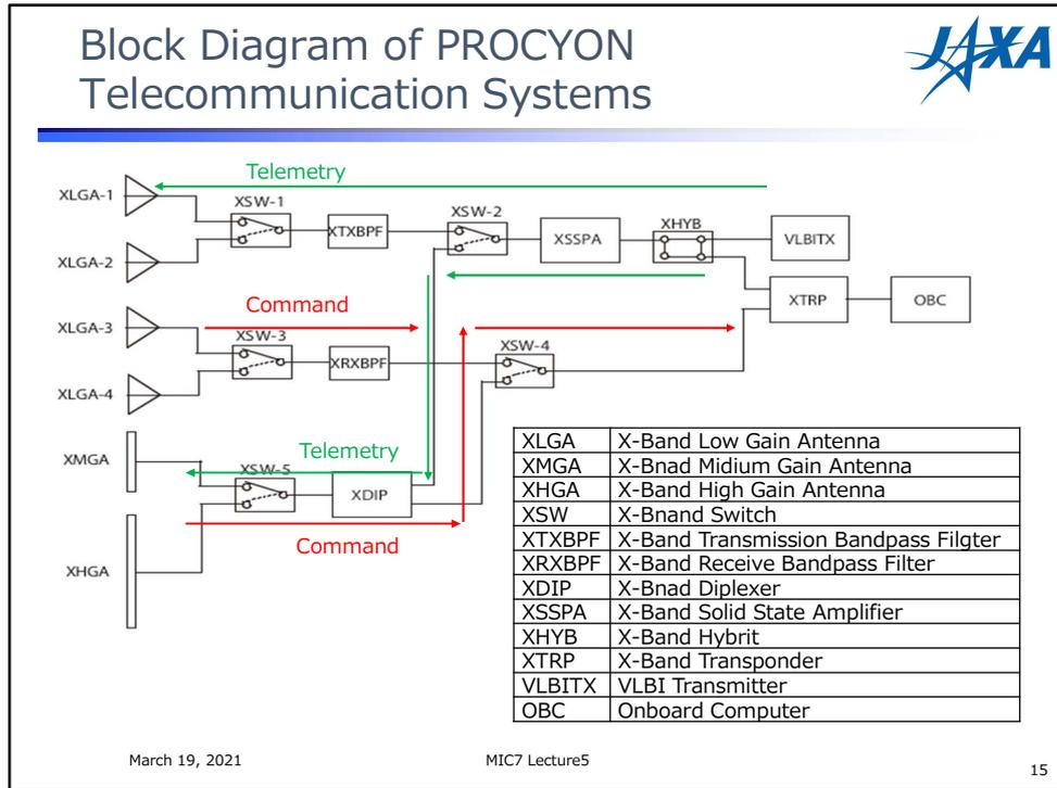
This slide shows a system diagram of the communication system installed in PROCYON. Looking at this diagram, we can see that the communication system consists of many components and is a collection of elemental technologies.
