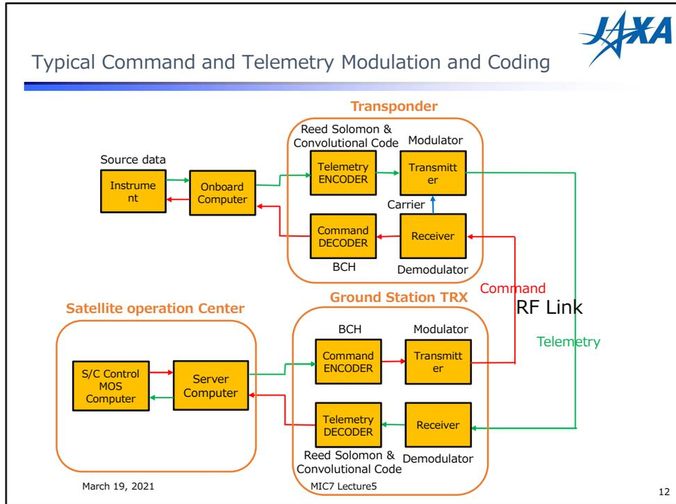
The transponder is responsible for receiving radio signals coming from the earth station, extracting commands and passing them to the onboard computer, while receiving telemetry from the satellite from the OBC and transmitting it to the earth station. The XTRP is called a transponder because it receives signals transmitted from the Earth and transmits them back to the Earth side in order to accurately determine the location of the satellite in space.
