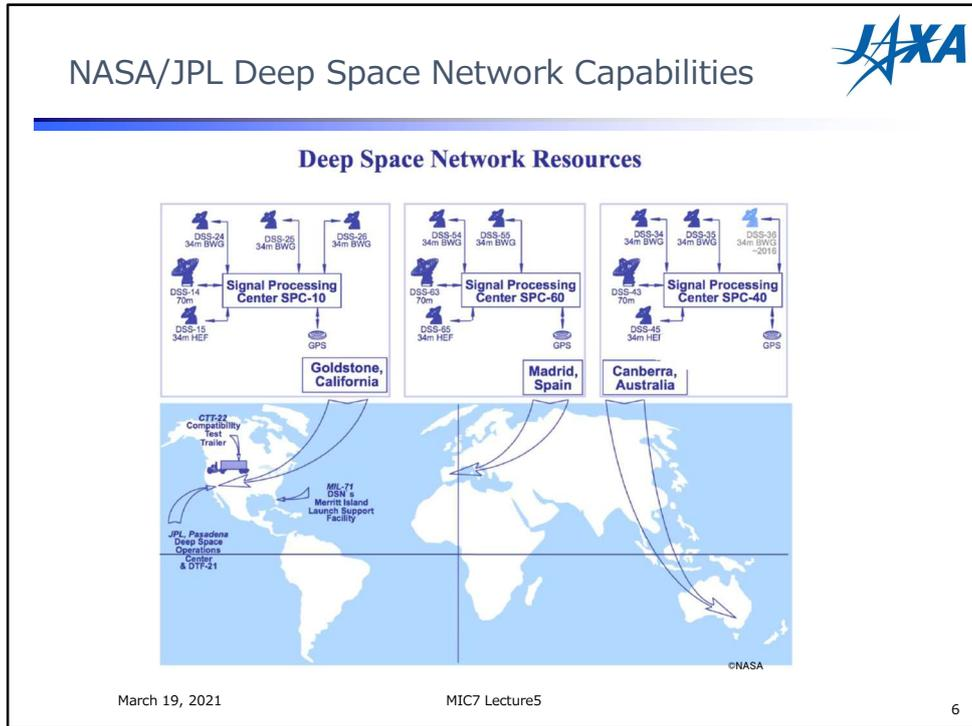
This slide shows the resources of the DSN worldwide: one 70-m antenna and four 34-m antennas in one complex, capable of operating more than 100 space exploration missions simultaneously.
