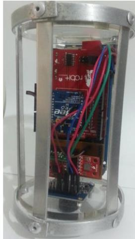
**Figure-3** The Can-Sat
