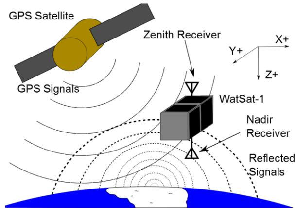
Figure 1: WatSat-1 Antenna Orientation
