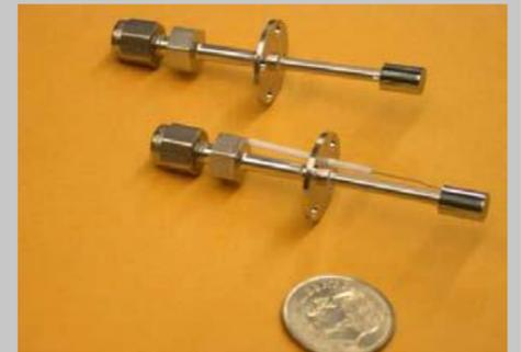
Figure 5: MiXI's Miniature Hollow Cathodes<sup>3</sup>
