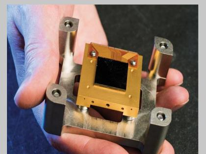
Figure 6: NEOCam Sensor<sup>4</sup>
